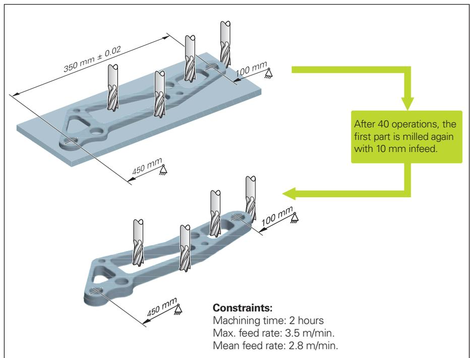
Figure 4 Manufacturing the coupling lever
