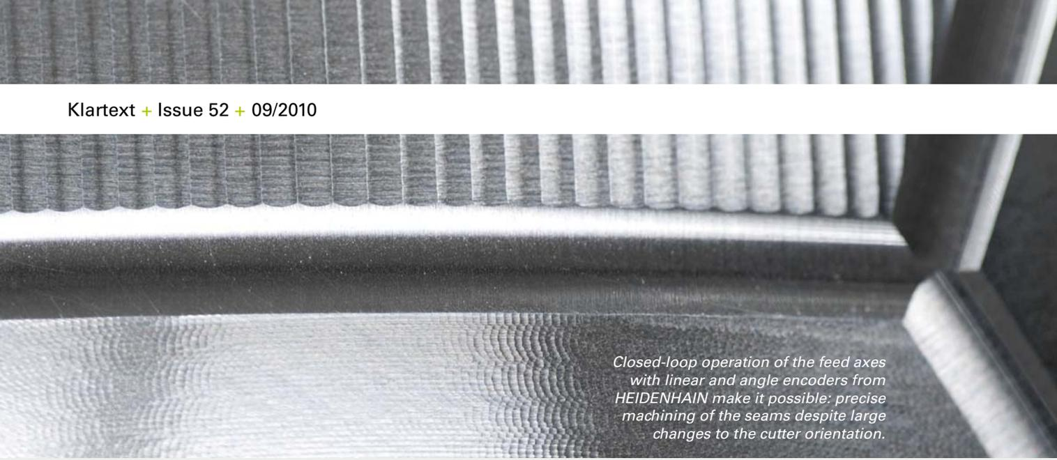
*Closed-loop operation of the feed axes with linear and angle encoders from HEIDENHAIN make it possible: precise machining of the seams despite large changes to the cutter orientation.*
